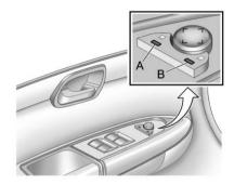
Controls for the outside power mirrors are located on the driver door armrest.
